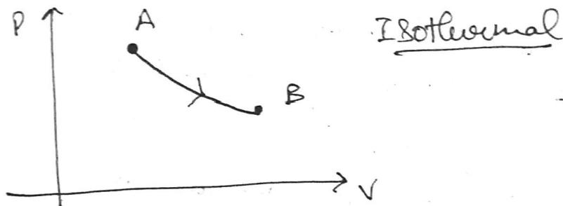
→ If we move sand from shelf to on piston, the system goes back quasistatically to same original state ( $A$ )
