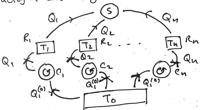
⊗  $C_1$  supplies  $Q_1$  heat to  $R_1$ , the same heat that it ~~loses to~~ loses to  $S$ , and so on to  $n$ .
