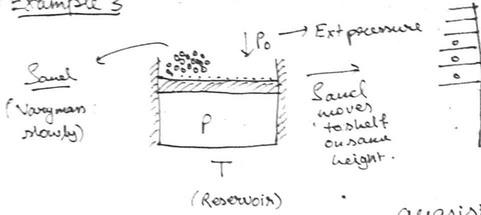
→ If we take sand off (gradually), the system moves up (taking heat from reservoir) quasistatically.
