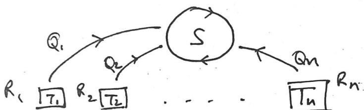
We introduce a reservoir with arbitrary temp  $T_0$ , and exactly  $n$  carnot engines.
